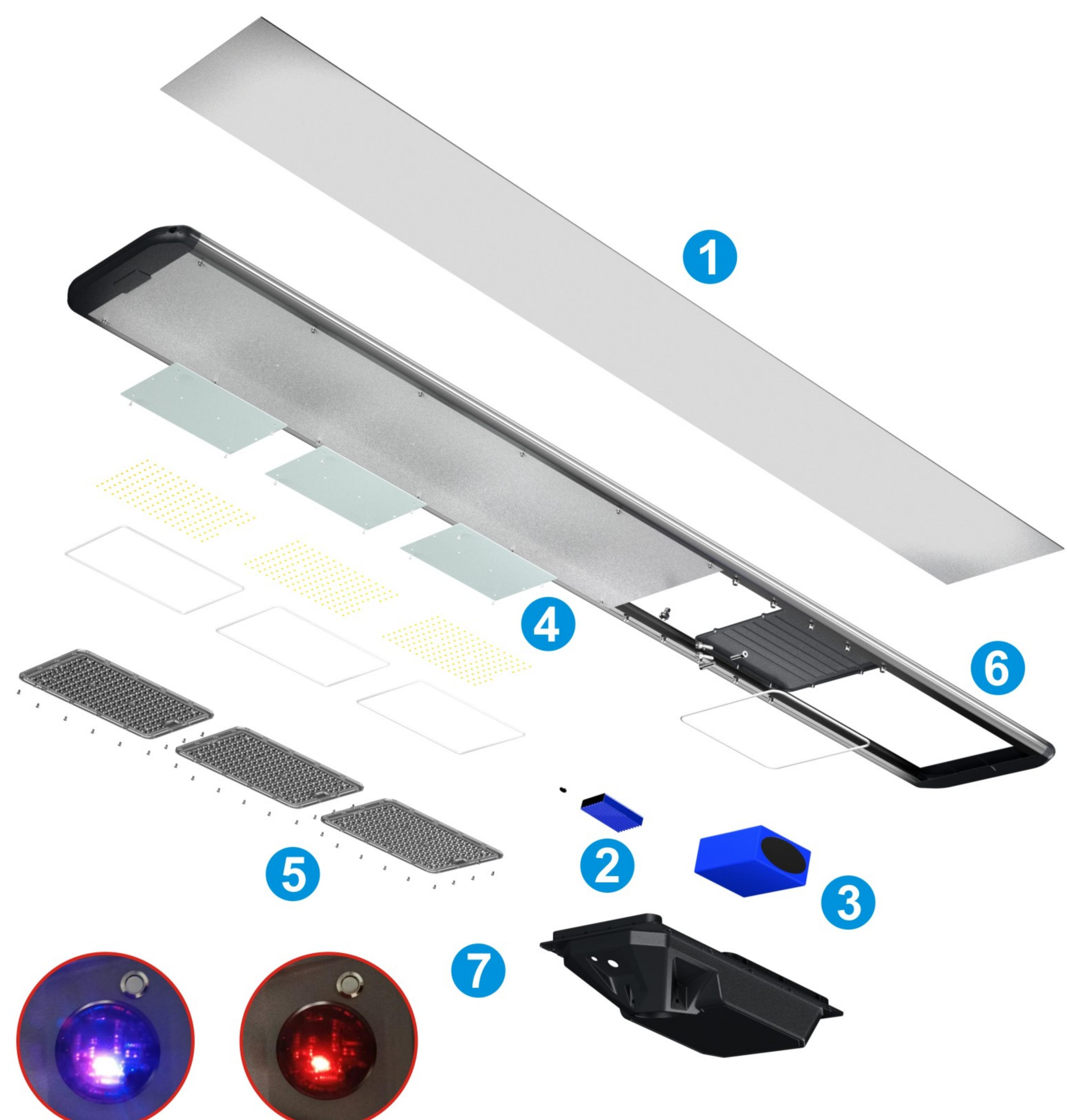
**1** Mono Solar Panel    **2** Control Module    **3** LifePo4 Battery
